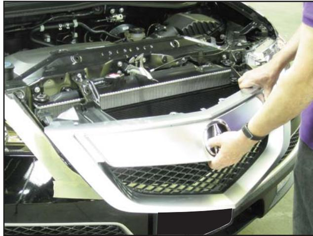
6. Once the lower push fasteners are removed, pull the grille forward and remove it from the bumper cover.
