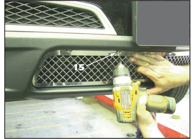
15. Align the **lower mesh grille assembly** into place and use a 1/16" drill bit to drill through the centers of the **mounting tabs** (as shown).
