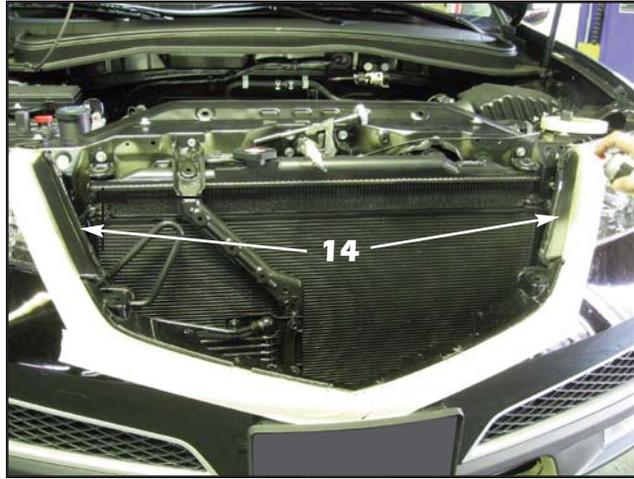
14. Paint everything inside the grille opening with flat or semi-gloss black paint that would be visible through the mesh grille, including the portions of the headlights scuffed in the previous step.
