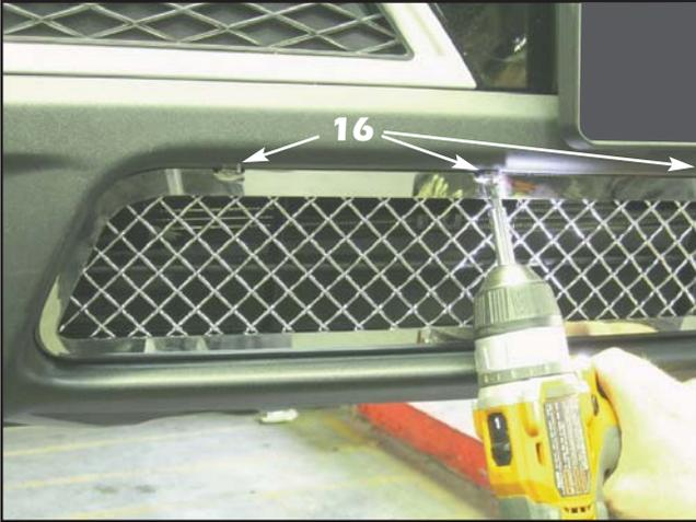
16. Install the supplied #6 x 1/2" Torx pin head screws through the **mounting tabs** and into the bumper cover.
