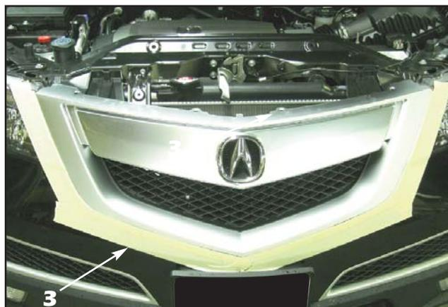
3. Apply several layers of masking tape around the perimeter of the factory grille to protect the painted bumper cover during the following grille removal procedure.
