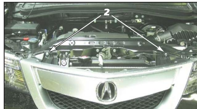
2. Remove the top 10mm fasteners retaining the grille (one per side).
