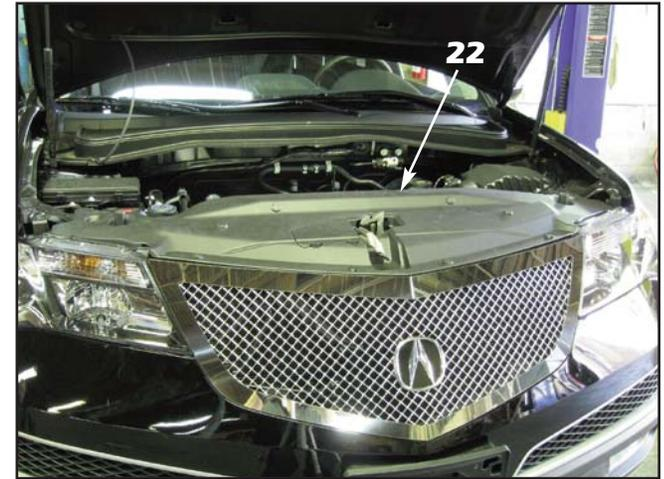
22. Reinstall the radiator support panel cover, reusing the factory hardware removed in **Step 1**.
