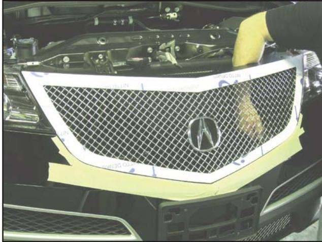
17. Align the **mesh grille** into place and reinstall the lower factory push pins removed in **Step 4**.
